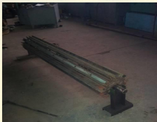
Figure 2. A rubber-plate separating drum prepared for the experiment
