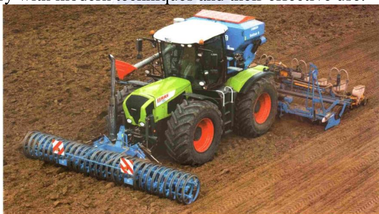
Figure 1. Soil loosening and seeding unit combined with Claas Xerion model tractor.
