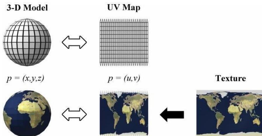
Fig. 1. Superimposing a two-dimensional texture on a three-dimensional object
