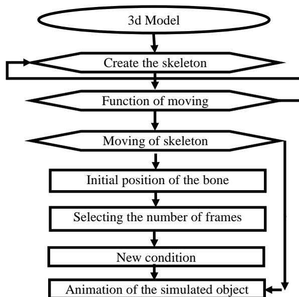
*Fig. 2 Block diagram of the 3D model animation process*
