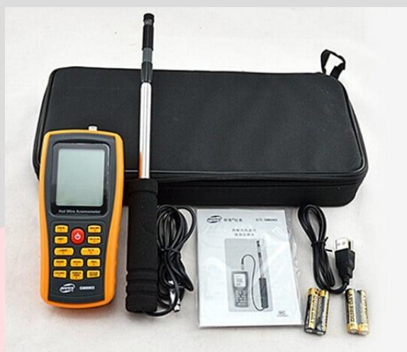
Figure 1. Benetech GM8903 Thermoanemometer for studying aerodynamic properties of fibres
