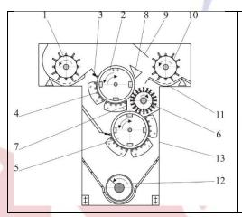
1, 10-a pile of drums, 2-saws strongly with the main drums, 3-ilashtiruvchi brush, 4-kolosnikli grill, 5-regenerasiyaya saws strongly drums, 6-brush echuvchi drums, 7-set, 8-yo'naltiriruvchi plate, 9-wall angle, 11-to'rli surface, 12-dirty shnekonthe 13-ramadan.
