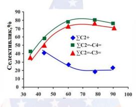
**T=340** °*C*, R = 0.1 MPa,  $V_{aral} = 1200h^{-1}$ . Raw material: 15% dimethyl ether +85%  $N_2$ Figure 1. Dependence of the selectivity of the reaction products in the Mg-Zr-Zn-B-HSZ catalyst on the amount of water vapor in the initial dimethyl ether:mixture
