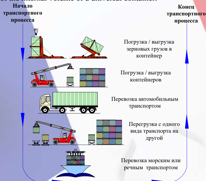
Rice. 6 - Scheme of intermodal transportation of bulk cargo in containers, in bulk (by road and water transport)
