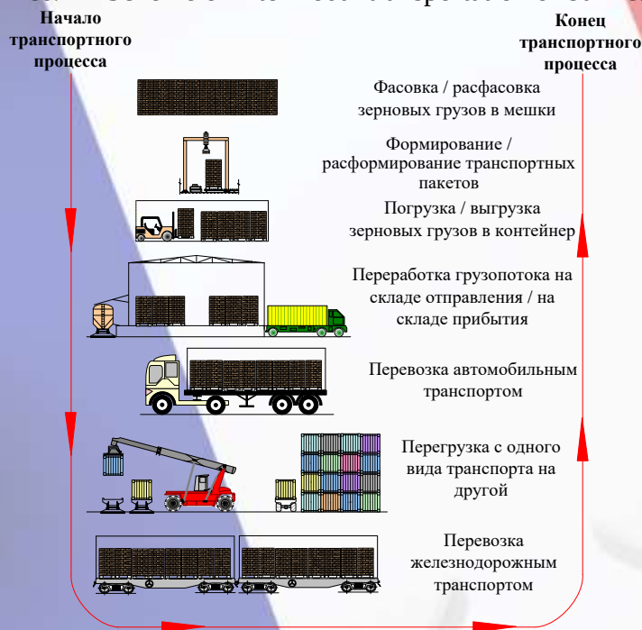
Rice. 2 - Scheme of intermodal transportation of bulk cargo in overpacks
